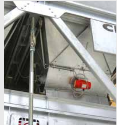
Electric vibrators and moisture probes (microwave or capacitive type) can be installed on very dosing cone.
