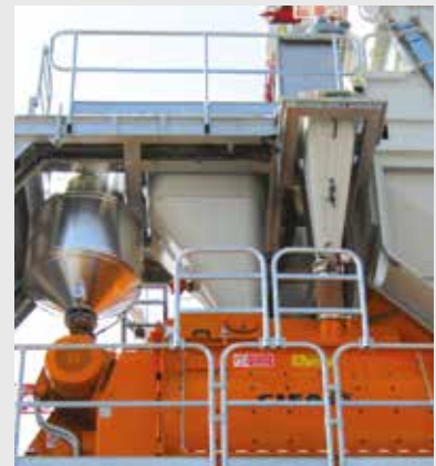
Micro silica weighing hopper.
