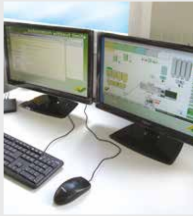
CIFAWIN automation control system including industrial computer.
