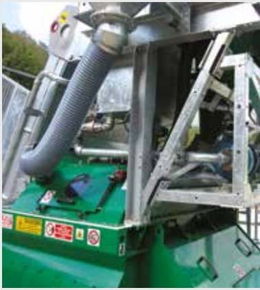
Mixer washing system with special pump and nozzles inside the tank.
