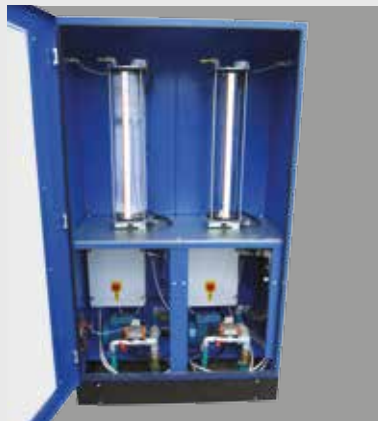
Chemical additives dosing system by weight.
