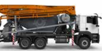
MK 24.4Z BOOM HEIGHT: 23,5 m BOOM SECTIONS: 3
