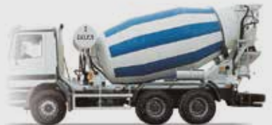
RY/SRY 1100 NOMINAL CAPACITY: 10 m³ with or without auxiliary engine - FOR ITALIAN MARKET ONLY
