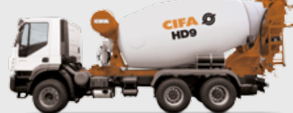
HD/HDA 9 NOMINAL CAPACITY: 9 m³ with or without auxiliary engine
