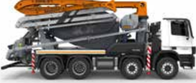
MK 25H BOOM HEIGHT: 24,2 m BOOM SECTIONS: 4
