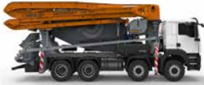
MK 32L BOOM HEIGHT: 31,2 m BOOM SECTIONS: 4
