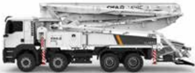
K41C BOOM HEIGHT: 40,1 m BOOM SECTIONS: 5
