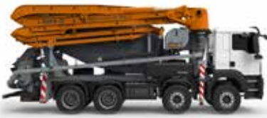
MK 28L-5'' BOOM HEIGHT: 28,1 m BOOM SECTIONS: 4
