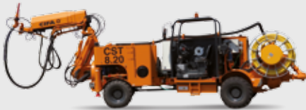
SHOTCRETE CST 8.20 THEORETICAL OUTPUT (MIN - MAX): 2 - 20 m³/h MAX PRESSURE ON CONCRETE: 65 bar
