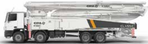
K56C BOOM HEIGHT: 56 m BOOM SECTIONS: 6
