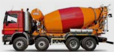
RY/SRY 1300 NOMINAL CAPACITY: 12 m³ with or without auxiliary engine - FOR ITALIAN MARKET ONLY
