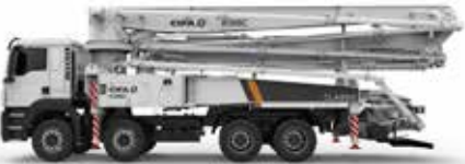
K38C BOOM HEIGHT: 37,6 m BOOM SECTIONS: 4
