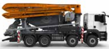
MK 28L-4'' BOOM HEIGHT: 28,1 m BOOM SECTIONS: 4
