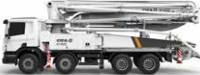
K40C BOOM HEIGHT: 39,5 m BOOM SECTIONS: 5
